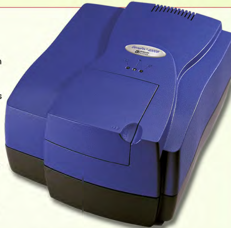
Fig. 31 The GenePix 4000B Microarray Scanner is used to scan Nimblegen and other arrays spotted in a 1" x 3" format at 5 \mu m -100 \mu m resolution (16-bit dynamic range).
